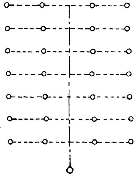
FIG. 4 TWO END-CENTRE WITH END FEED
