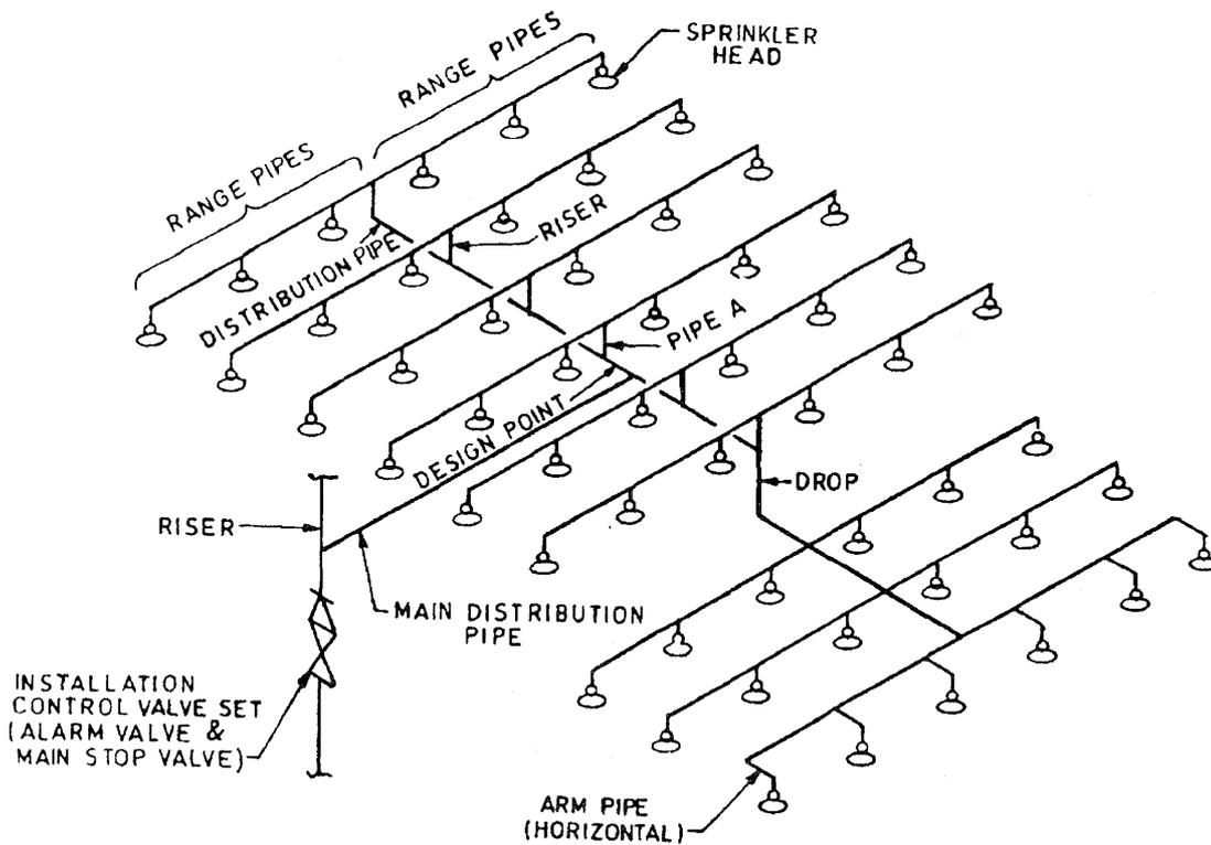
FIG. 1 MAIN ELEMENTS OF A SPRINKLER INSTALLATION
