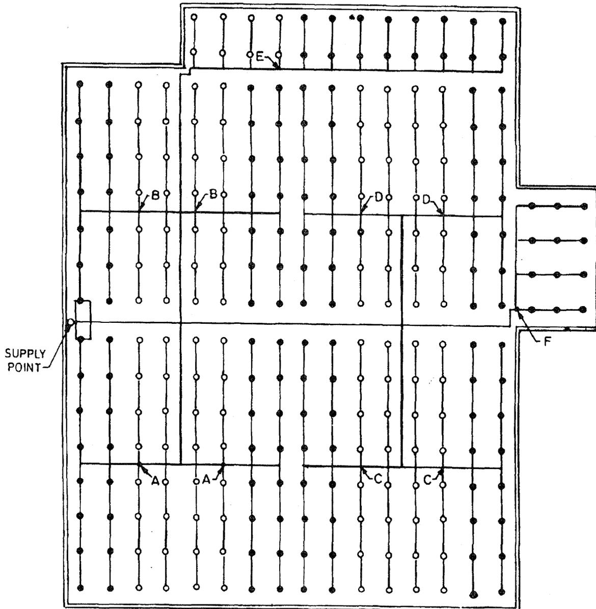
FIG. 21 DESIGN POINTS IN AN OH INSTALLATION
