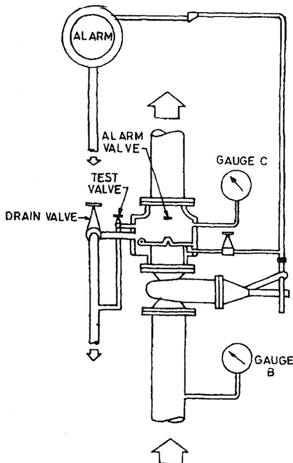
FIG. 29 SPRINKLER INSTALLATION VALVE ASSEMBLY
