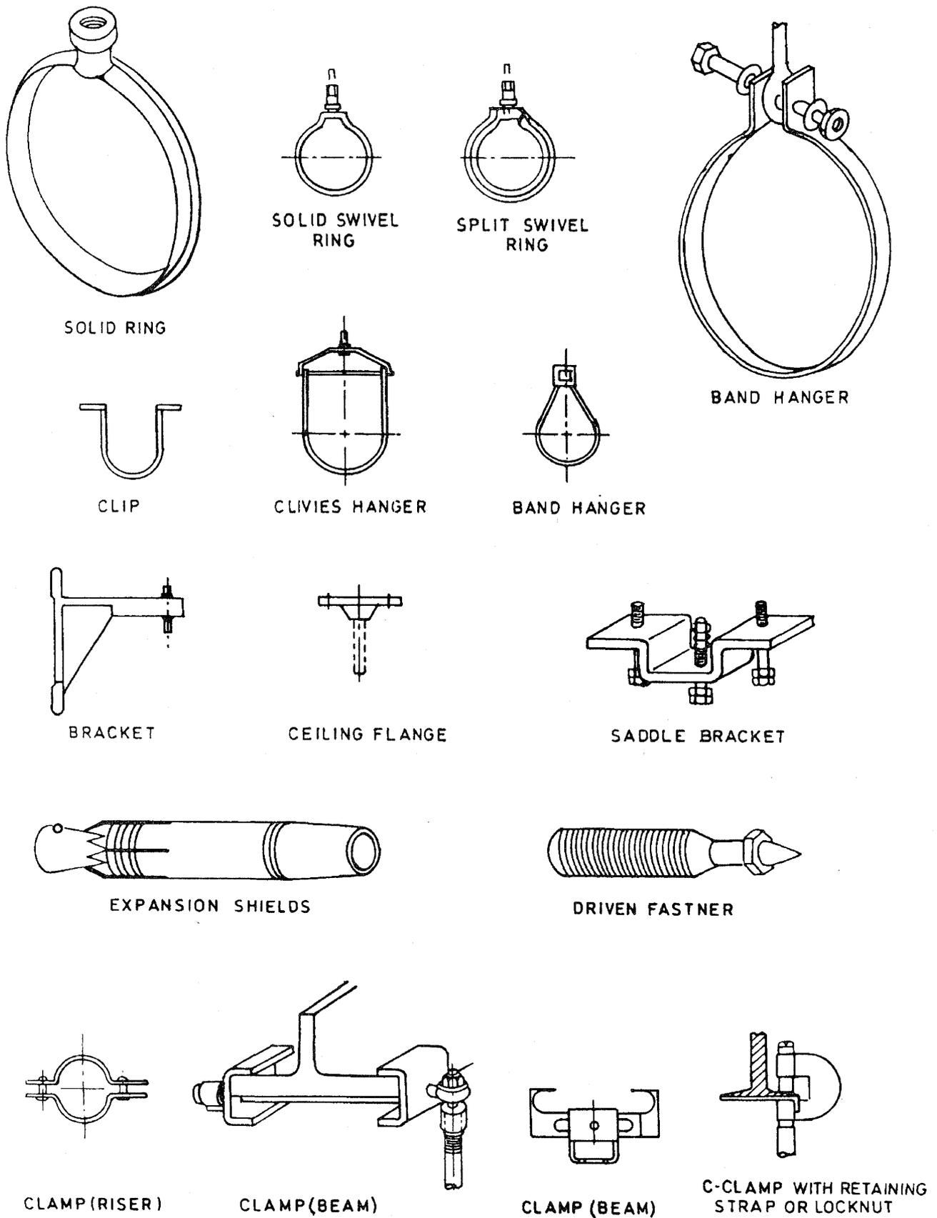
FIG. 15 COMMON TYPES OF PIPE HANGER EQUIPMENT
