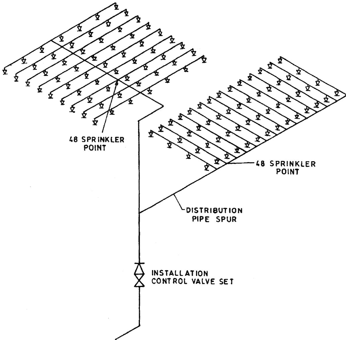
FIG. 22 DESIGN POINTS IN HIGH HAZARD INSTALLATION WITH PIPEWORK SIZED FROM TABLES 32 AND 33
